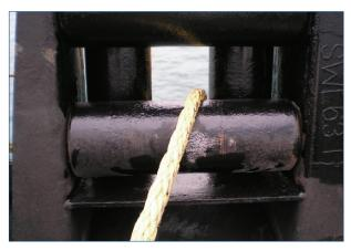
This cost savings can be a big advantage when converting a vessel from wire to HMPE rope. Conversion is a costly expenditure and installing new closed chocks, instead of new roller chocks, can provide significant savings.
